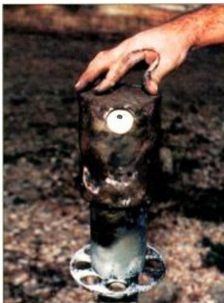
Dust-laden moisture forms a conductive path, as indicated by the burned Teflon. As the path arcs over, transmission line failure occurs.
