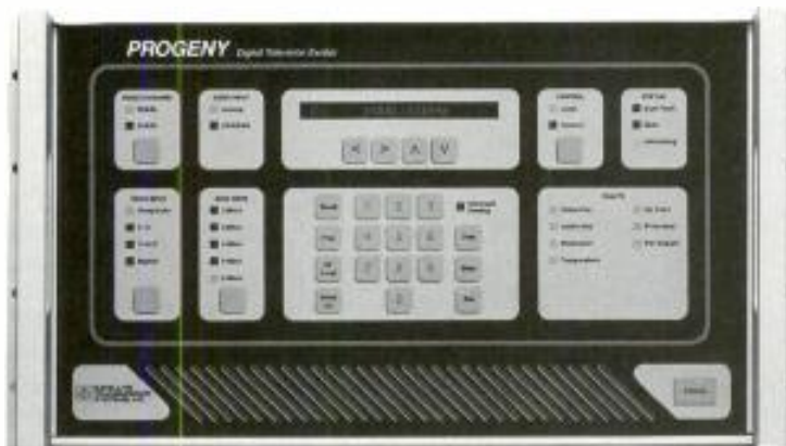
Digital TV exciter from Satellite Transmission Systems.
